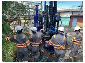
Guyana Shorebase Inc. (GYSBI): C.B. & Associates Inc. provided geotechnical services for the purpose of establishing representative soil parameters for a revetment design. Cone penetration testing (CPT), and standard penetration testing (SPT) were executed to classify the soil strata and to establish parameters for the design.
