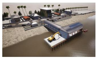
investigation; hydrographic surveys, geotechnical data collection, hydrologic and hydraulic modelling, and detailed designs. The finalised wharf design consisted of prestressed/precast piles and pre-cast beams and slabs and a steel-framed superstructure.
