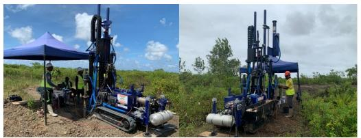
**GUYANA POWER & LIGHT (GPL):** C.B. & Associates Inc., provided geotechnical services for the purpose of establishing representative soil parameters for the development of photovoltaic solar farms on the Essequibo Coast and Berbice. Cone penetration testing (CPT), and standard penetration testing (SPT) were executed to classify the soil strata and to establish parameters for the design.
